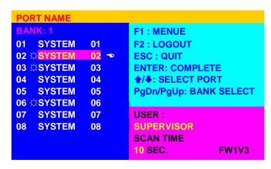
Use the cursor keys to select the computers connected on bank 1. Select the computer by pressing the ENTER key. This symbol indicates all active computers connected. Computers connected not showing this symbol may either be switched off or in a standby mode. To access ports between 9...16 simply scroll down below port 8.
